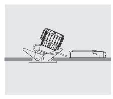
4. Adjust the angle required. Installation complete.
