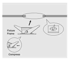
1. Cutout and compress spring plates to insert fixture frame to ceiling.
